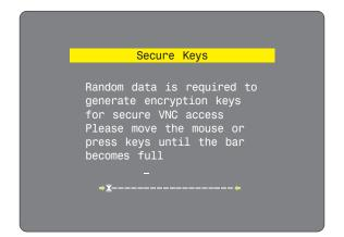
With every mouse move and keypress, the single dash will move across the screen (unless the same key is pressed repeatedly). Periodically, a new star character will be added to the bar as the random data is accepted as part of the new encryption key. When the bar is full, the final encryption keys for your CPU IP will be created – this process takes roughly 30 to 40 seconds.
